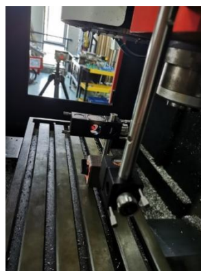
Fig 6: The Collimation of the linear mirror sets with laser beams
