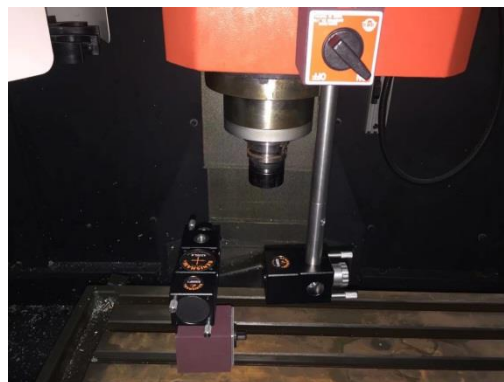
Fig 4: The Installation diagram of linear mirror set
