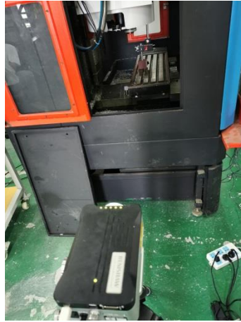
Fig 3: The installation diagram of the tripod and the laser
