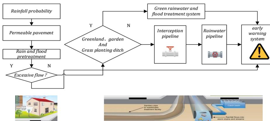
Fig 4: Green rain and flood management system
