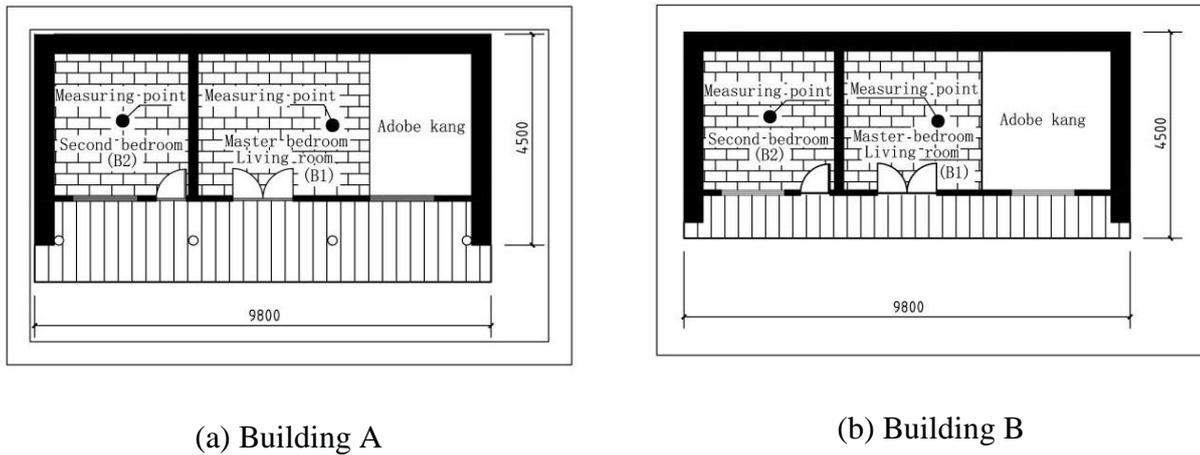
Fig 2 Layout of building and measuring points
