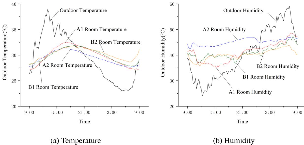
Fig 4 Temperature and humidity changes in summer
