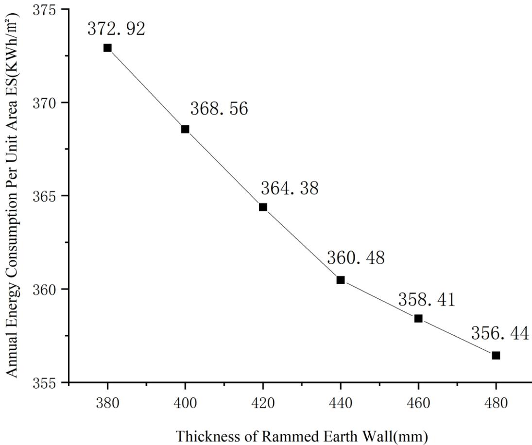
(e) Thickness of rammed earth wall
