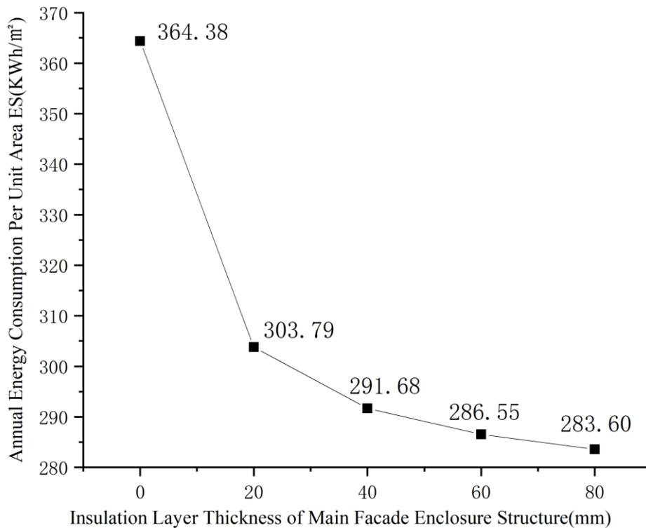
(a) Insulation layer thickness of main facade enclosure structure
