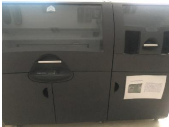
Fig 1: The full color 3D printer of Projet CJP 660 Pro
