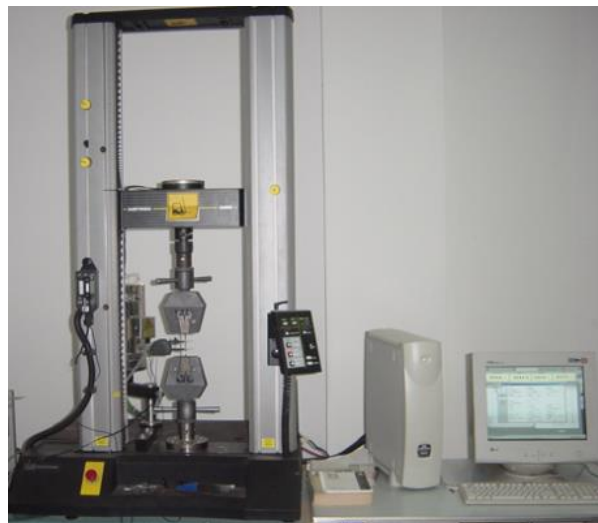
Fig 2: The mechanical test platform of Instron 3367
