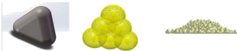
(c) Filling and stacking effects of triangular-like particles
