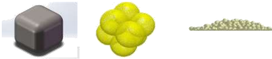
(b) Filling and stacking effects of quasi-cubic particles
