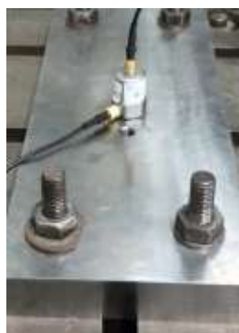
Fig 5. In-situ calibration of accelerometer with vibration isolation foundation
