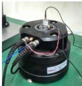
Fig 3. The sensitivity of the piezoelectric accelerometer was calibrated by comparison method.
