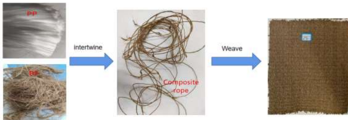
Fig 3: Preparation of BF/PP braided material
