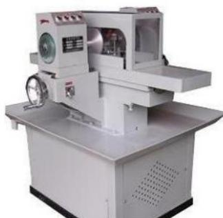
**Fig 2: SHM-200 double-end grinding stone machine**
