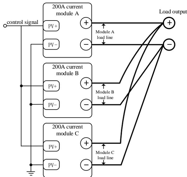
Fig 4: Current power amplifier power supply
