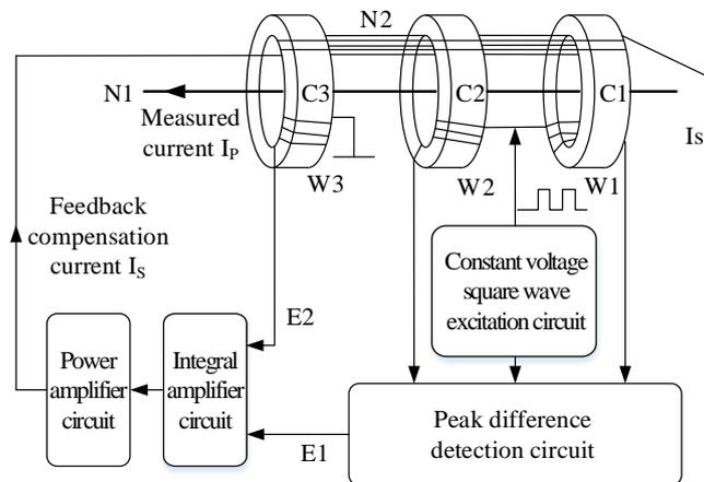
Fig 3: Principle block diagram of zero flux sensor E1 E2
