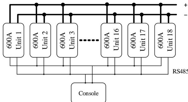
Fig 1: Structure Diagram of 10kA Standard DC Constant Current Source
