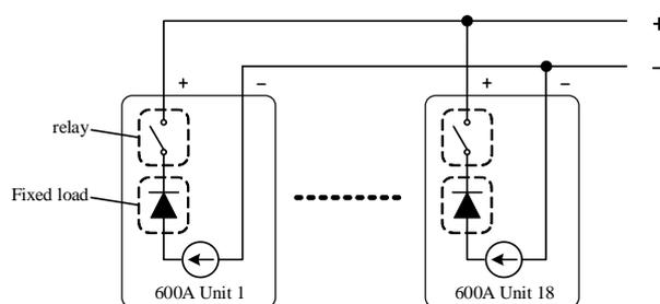
Fig 5: Parallel Structure Diagram of Constant Current Source
