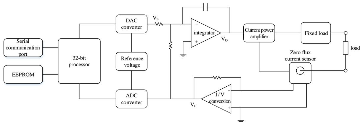
Fig 2: Principle block diagram of 600A constant current source circuit
