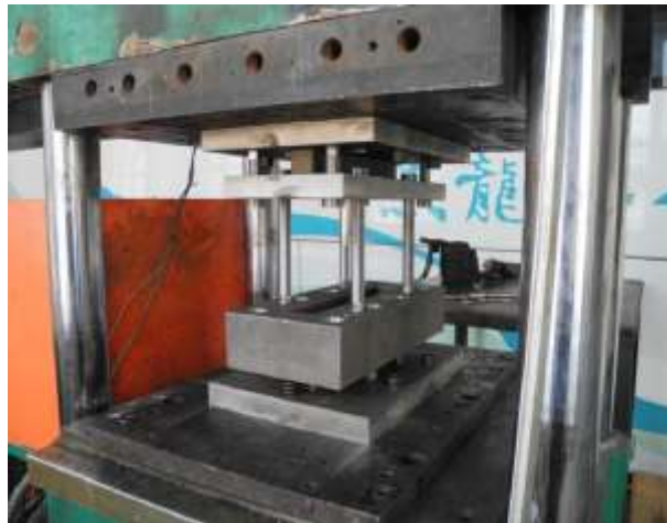
Fig 2: Corn Porous Seedling Bowl Compression Molding Mould
