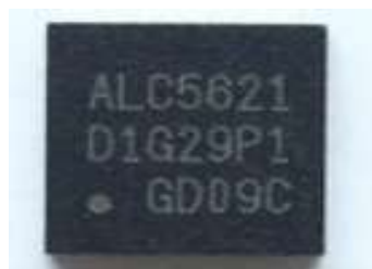
Fig 10: Physical Picture of ALC5621 Chip
