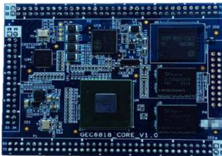
Fig 5: Front Side of Physical Picture of S5P6818 Core Chip
