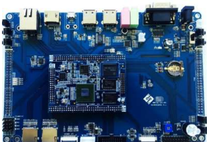
Fig 7: Physical Picture of S5P6818 Demo Board
