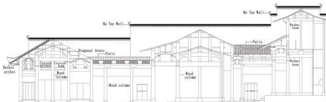
Fig 2: Schematic diagram of the patio of Chengzhi Hall in Hongcun (“o” indicates the load-bearing wooden pillars)
