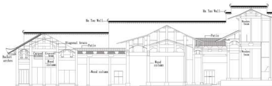
Fig 1: Cross-section of the wooden structure of Xuzhi Hall
