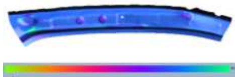
Fig 7: Blank thinning rate distribution diagram.
