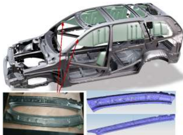
Fig 1: Physical drawing of high strength steel plate for vehicle.
