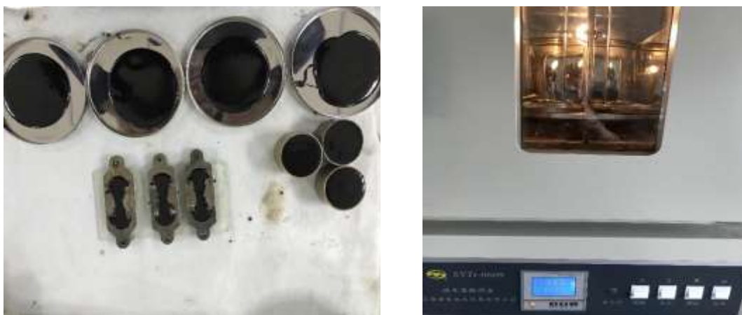
Fig 14 Thin-film oven asphalt aging test
