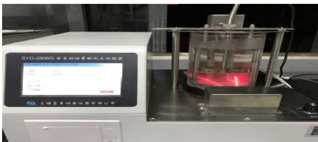
Fig 1 Asphalt softening point test
