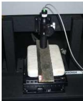
Fig 2: PS50 profiler for surface measurement
