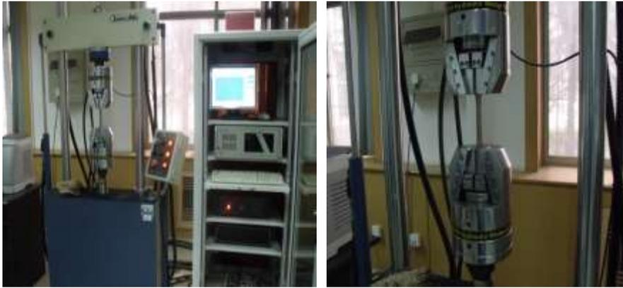
Fig 3: Fatigue test setup
