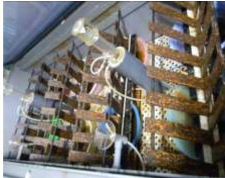
Fig 1: Placement of test pieces in the salt spray box
