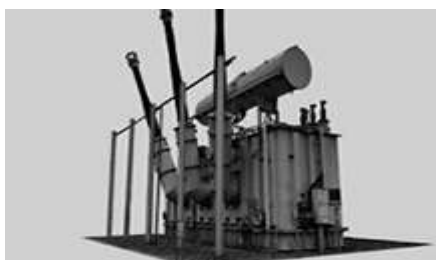
Fig.1 The 3d model of oil-immersed transformer
