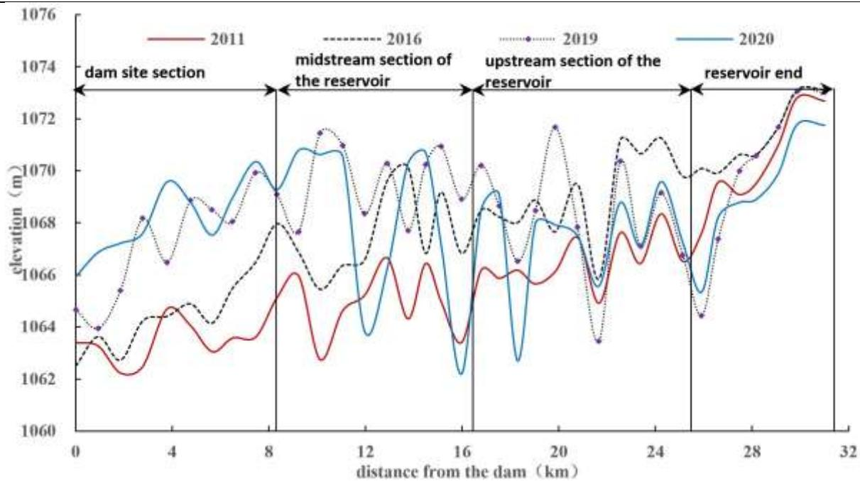
Fig 9: Thalweg profile change diagram of Haibowan Reservoir
