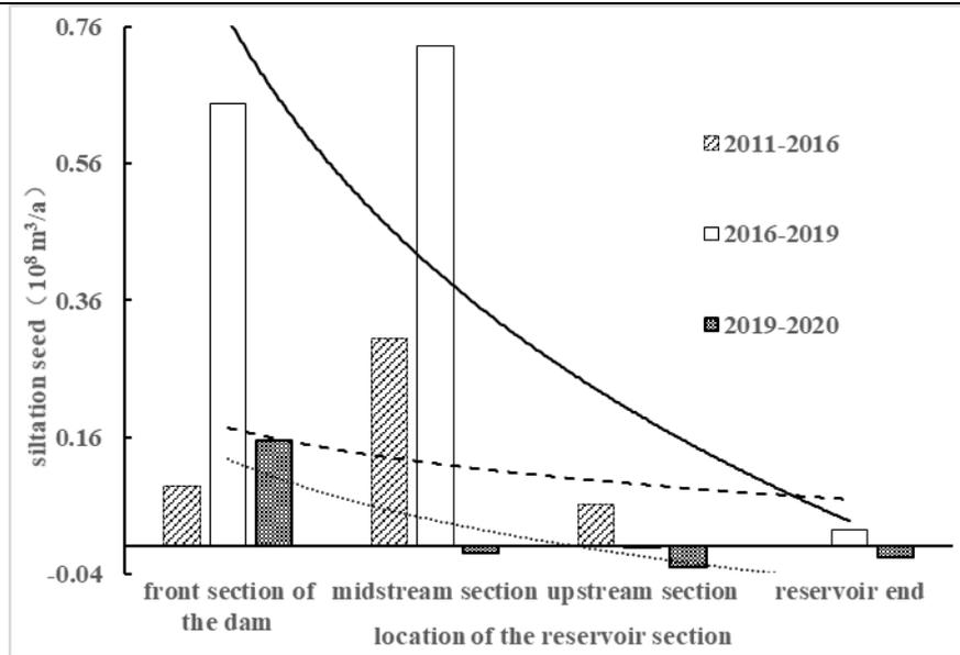
Fig 7: Siltation speed changes of Haibowan reservoir area (2014-2020)
