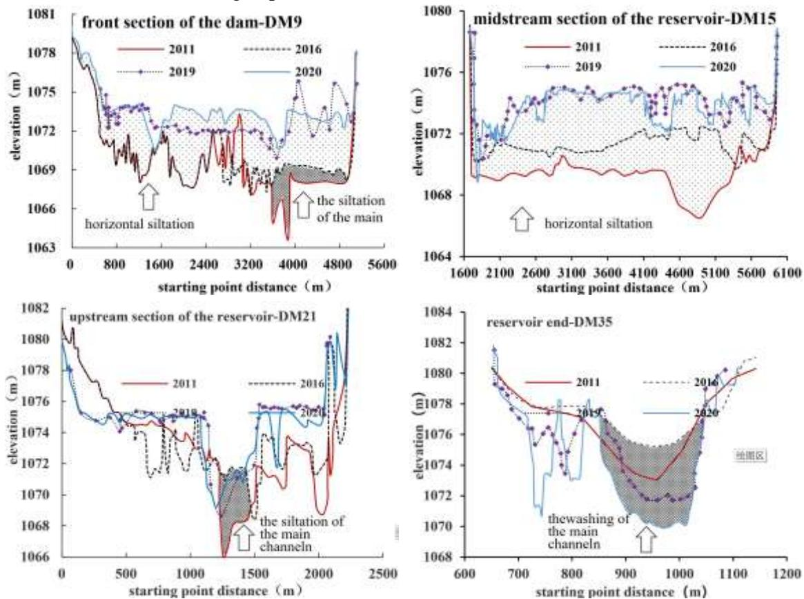
Fig 8: Typical cross-sectional plotting of the reservoir
