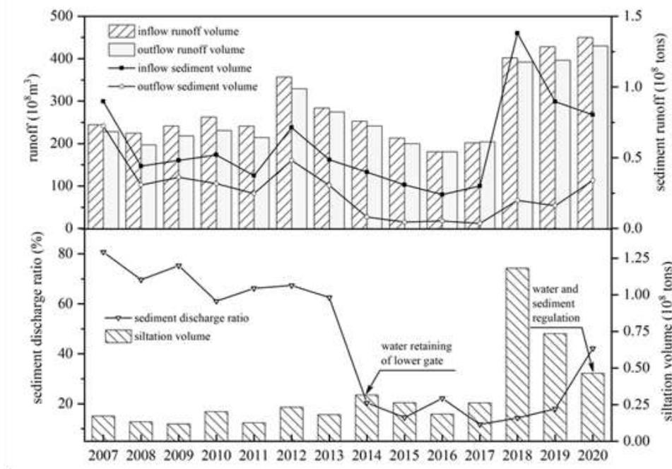
Fig 4: Inflow and outflow water and sediment conditions, siltation volume and sediment discharge ratio of Haibowan Reservoir over the years
