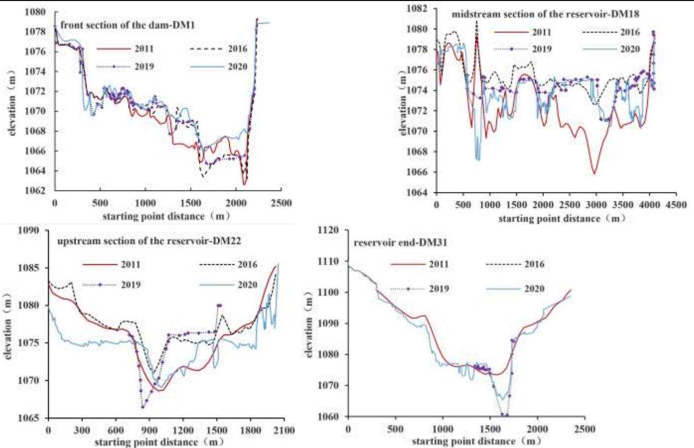
Fig 6: Typographic changes of the typical sections in Haibowan Reservoir (2014-2020)
