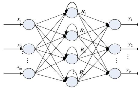
Fig: 3 Schematic diagram of Elman neural network
