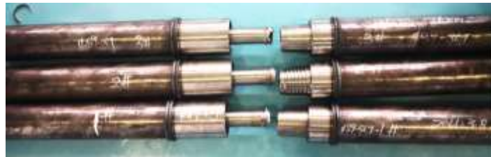
Fig 8: Fracture morphology of tendon rod
