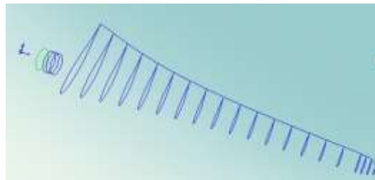
Fig 4: root circle curve of wind turbine blade
