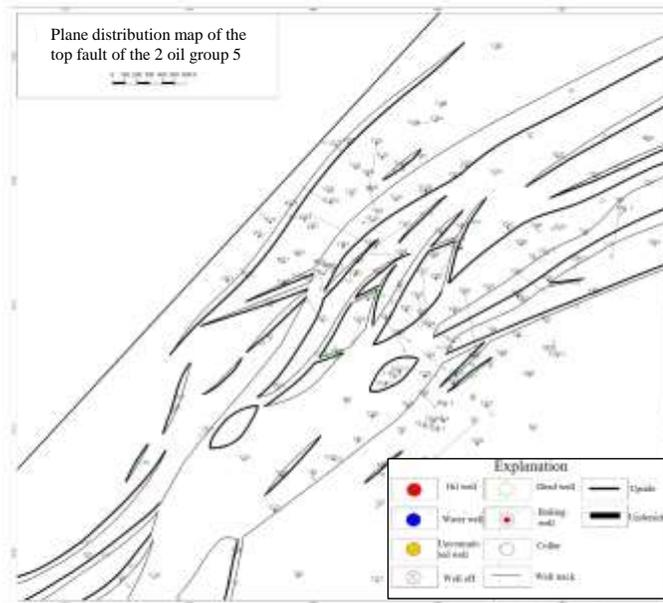
Fig 6: plane distribution characteristics of complex fault block groups of compound graben type
