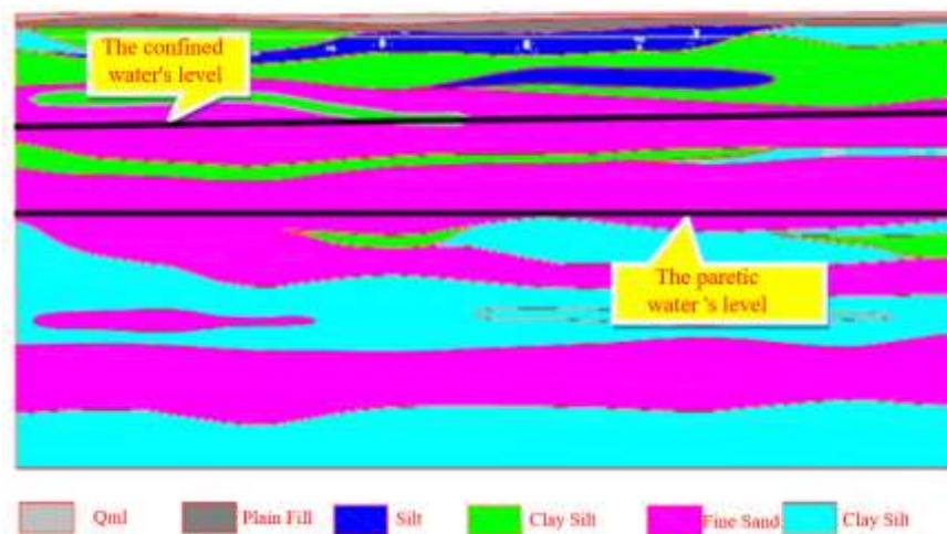
Fig 3: Geological section of the enclosure
