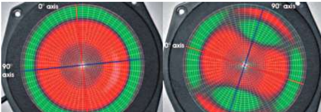
Figure 9 Operating deflection shape at 10kHz
