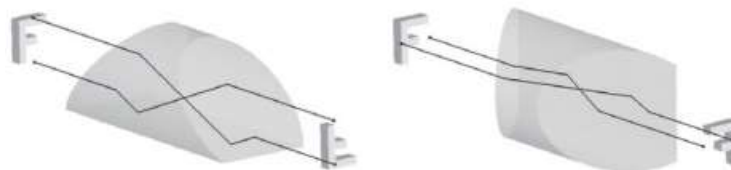
Figure 4 Working principle of Dove prism
