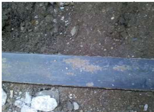
Fig 3: The corroded grounding electrode outside the grounding grid.
