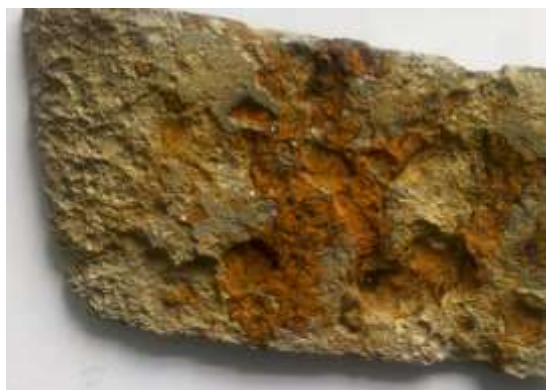
Fig 3: The corroded grounding electrode outside the grounding grid.
