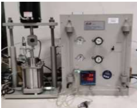
Fig 2: Pressure plate apparatus used in the ATT
