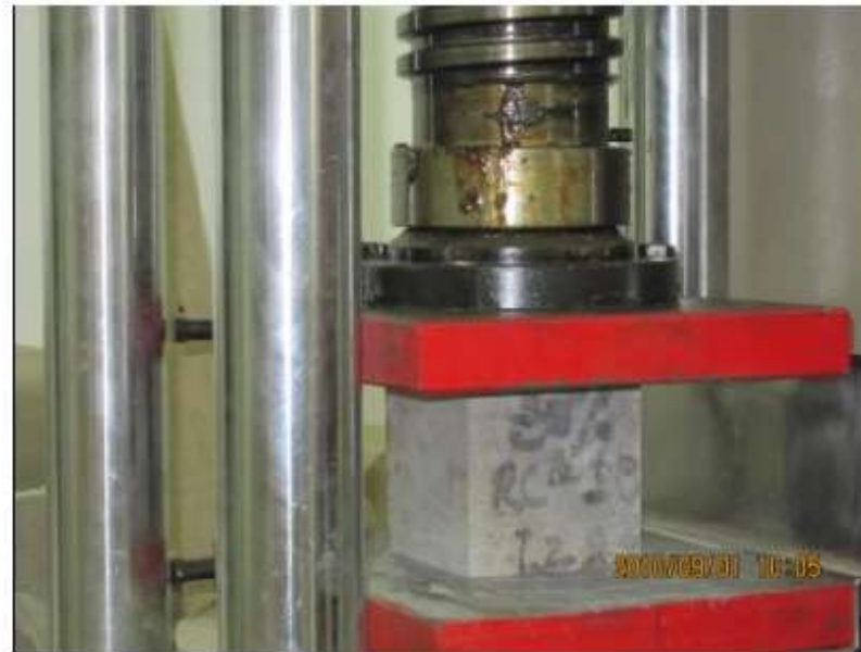
Fig 1: Cubic compressive strength test
