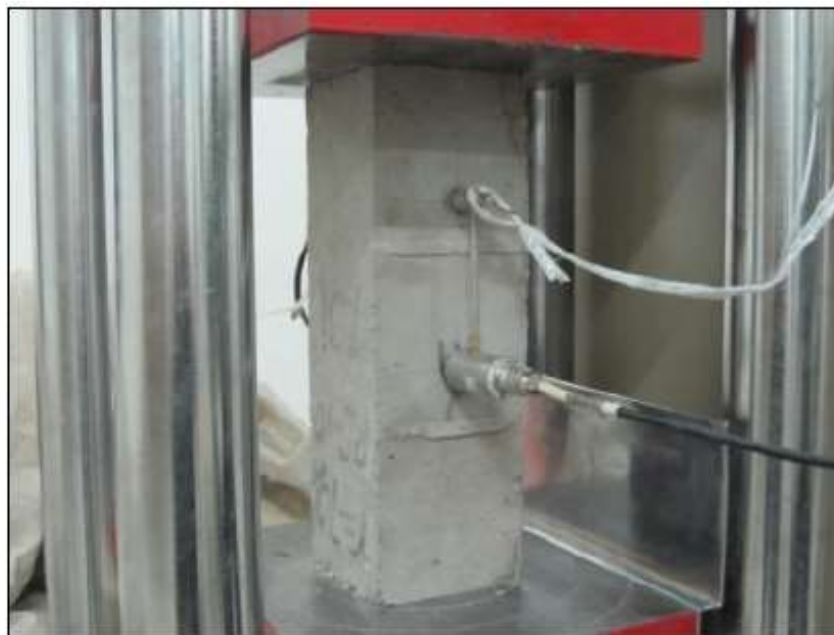
Fig 2: Compressive strength test of prism
