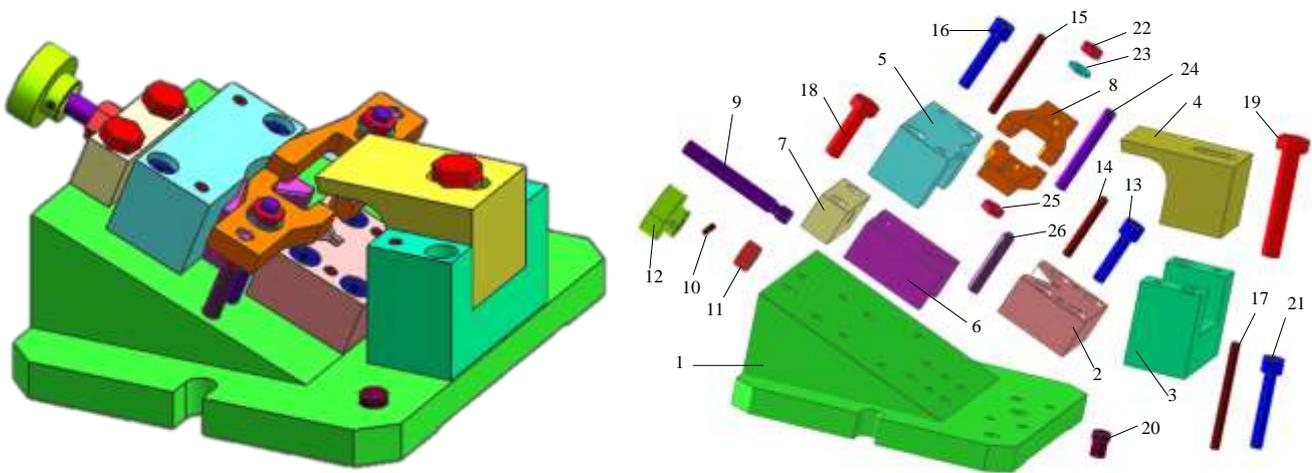
1-Body 2-V block 3 - Guide plate 4 - Pressing block 5 - Guide plate 6 - Pressing plate 7 - Plate 8 - Pressboard
