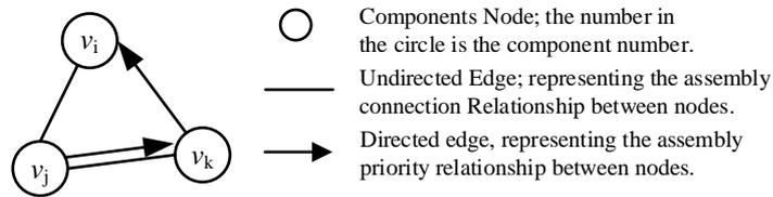
Fig 1: Basic elements for building models
