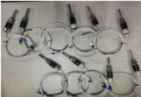
Fig 2: Pt100 temperature sensor
