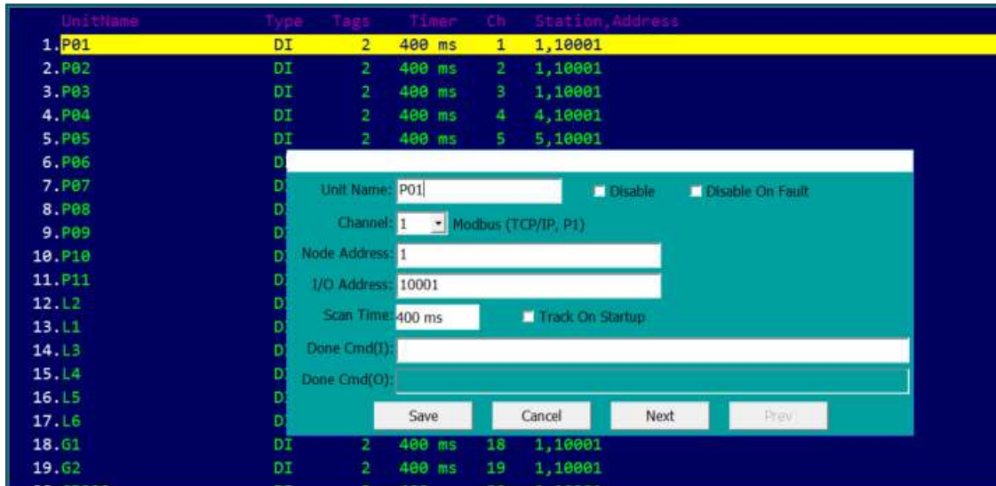
Fig 6: Receive signal setting interface
