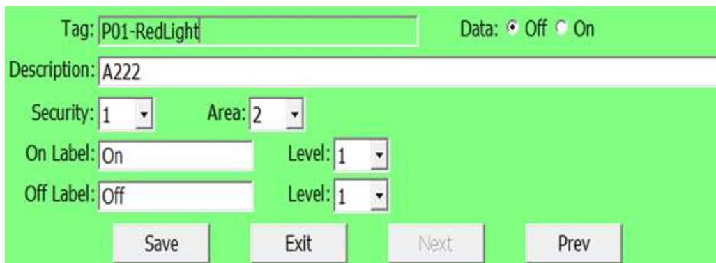
Fig 8: Machine operation signal setting(On once to start operation, Off once to stop operation)
