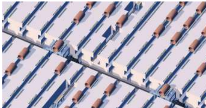
Fig. 6 partial diagram of multi multi-car conveying system in cold rolling intermediate Depot
